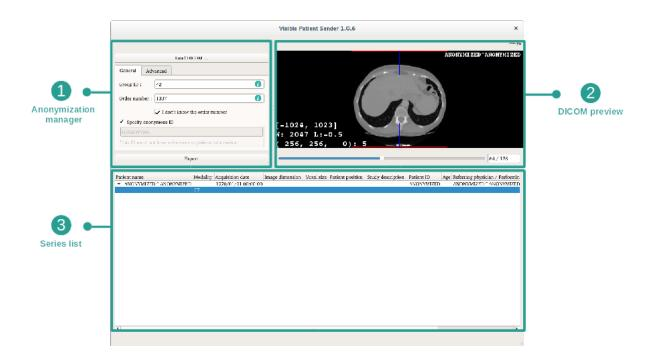
This software is composed of three main parts. The first one on the upper left corner is dedicated to the management of the anonymization process. The second one on the right side is a preview of the loaded DICOM files. The final one on the bottom is the list of the loaded series.
