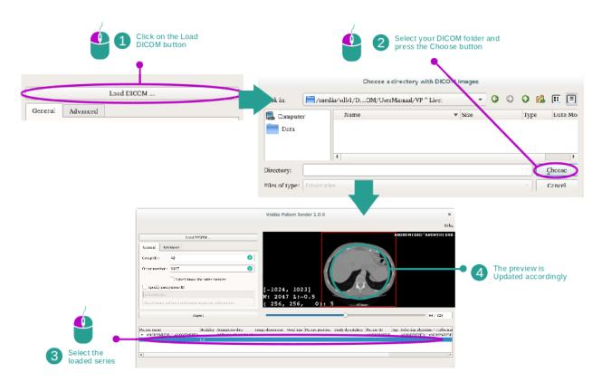
The first step to anonymize DICOM data is to load it into the Sender software. To do so, click "Load DICOM". Once loaded, the series is displayed on the list at the bottom of the view. You can then preview the series by selecting it in the list.
